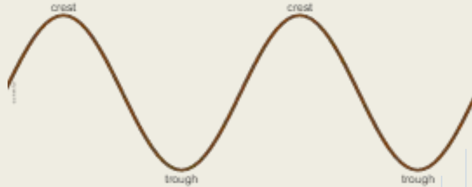
a transverse wave in a one-dimensional medium
